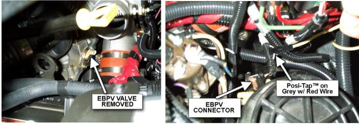
**NOTE:** After installation, ensure to replace the intercooler hose and clamps. Reattach the MAP sensor hose and wiring connector. Check all connections for security and tightness and secure all wiring to ensure they are out of the way of moving and heated items.
