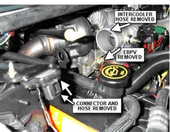
For ease of access and hook up, remove the connector from the EBP Valve and pull the wiring through and underneath to the front of the intake Y-plenum. This will allow access to install a Posi-Tap $^{\text{TM}}$  or Connector harness.
